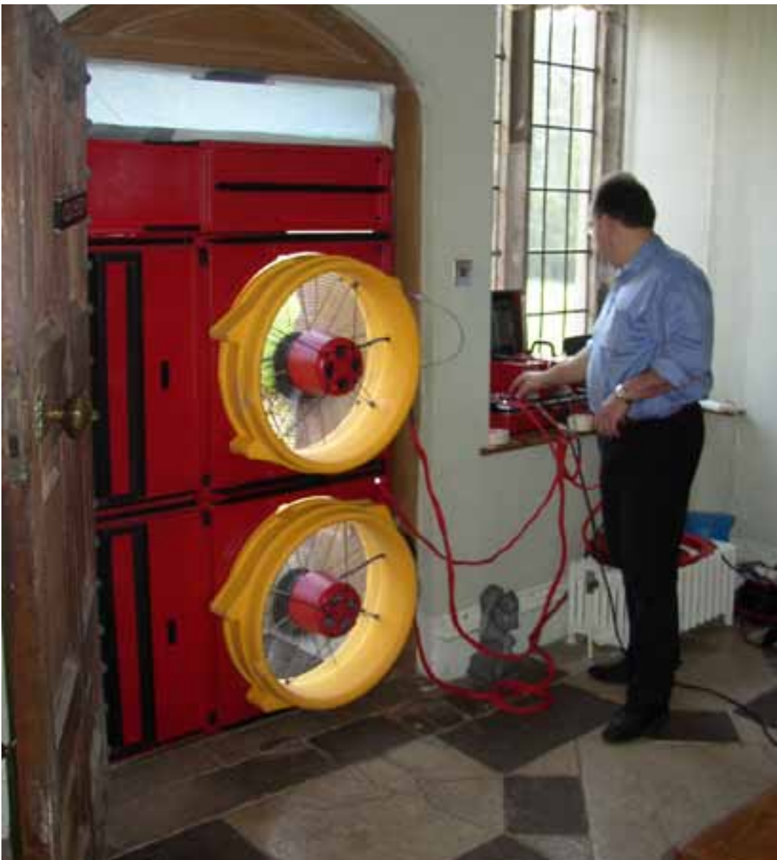
06 A fan pressurisation test is the most effective way of quantifying the amount of air infiltration and locating draughts that may not be immediately evident © Oxley Conservation
