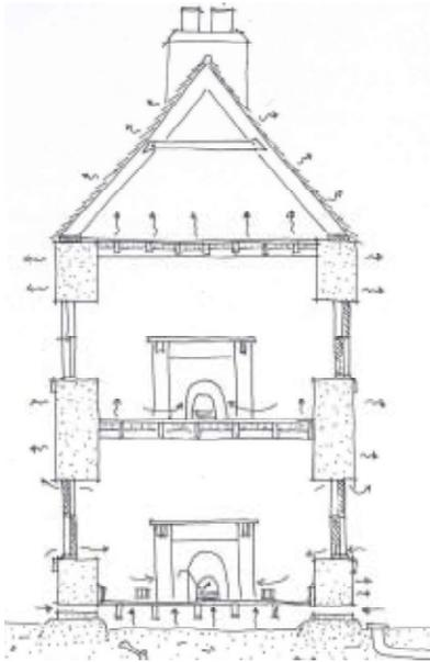
*Fig 1. Airflow and moisture movement in a traditionally built house.*
